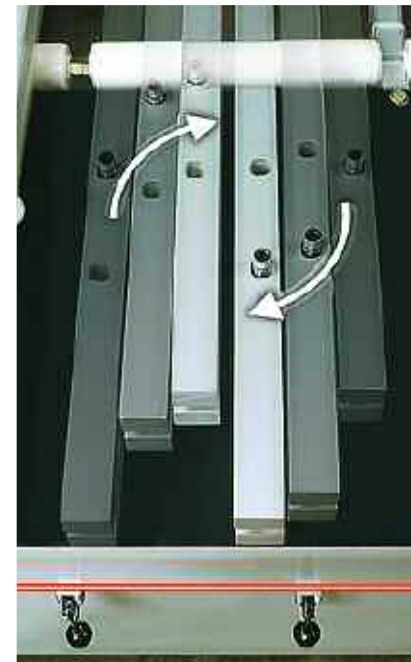
Air-activated, self-centering clamps for fixturing posts
