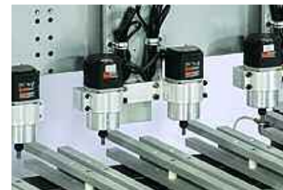
Fixture and machine multiple posts at a time. (Other router spindles available.)
